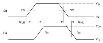
**WAVEFORM 1 - PROPAGATION DELAYS**  $t_R = t_F = 2.0$ ns, 10% to 90%; f = 1MHz;  $t_W = 500$ ns
