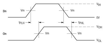
WAVEFORM 4 – PROPAGATION DELAYS  $t_R = t_F = 2.0 ns, 10\%$  to 90%;  $f = 1 MHz; t_W = 500 ns$
