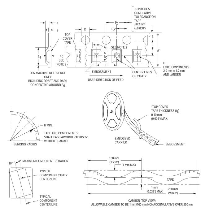
Figure 9. Carrier Tape Specifications
